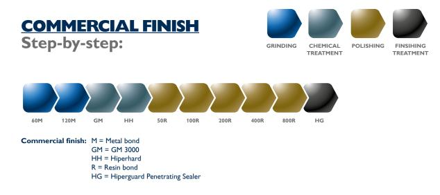
Note: When polishing concrete, we do not recommend grinding higher than 120 grit metal bond tools.
